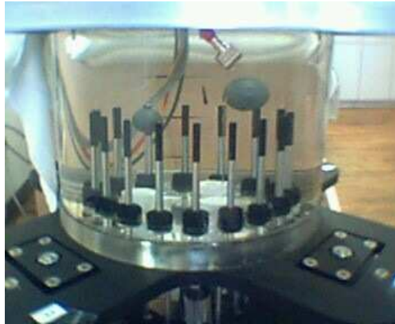
Figure 5.22: Experimental setup for the sphere phantom measurement.
