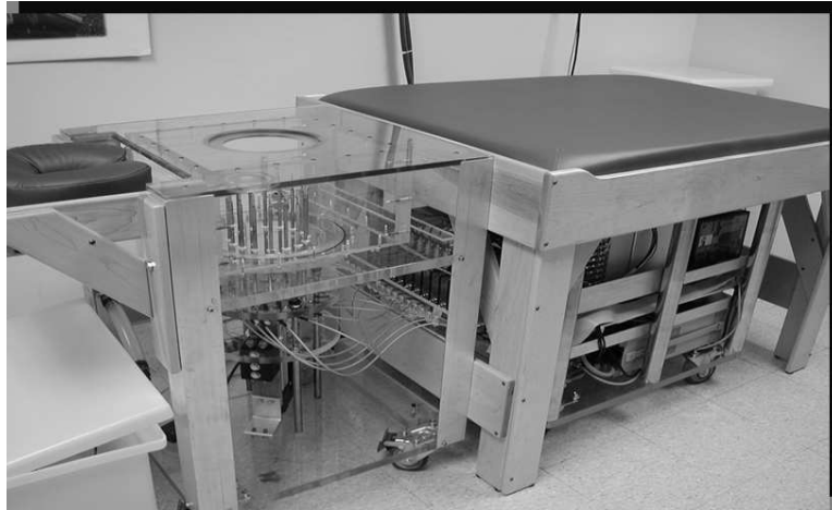
Figure 1.7: Photograph of the second generation microwave imaging system at Dartmouth College
